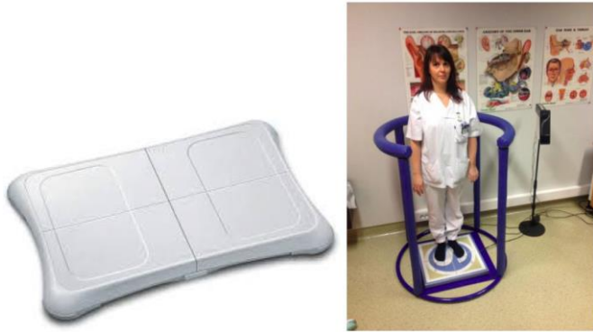
Fig 1. Wii Balance Board (WBB) on the left and force platform on the right at the Norwegian National Advisory Unit on Vestibular Disorders, Haukeland University Hospital, Bergen, Norway.
